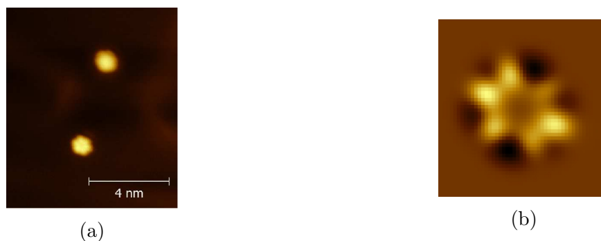
Figure 1.6: Experimental STM images of C_{60} on Au(111) obtained near zero bias. The single C_{60} in (b) is Laplace filtered. [23]
